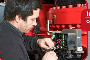
The commissioning of a crane vehicle requires the adherence of the German traffic regulations (StVZO) and the CE-certfication as well as the thorough assessment i.e. by a TÜV SÜD expert. By safety checking, testing the vehicle's carrying capacity and also proof-loading, it is ensured that the crane meets the legal requirements. A test seal and an entry written into the crane test and inspection booklet verifies that it is safe to use.
